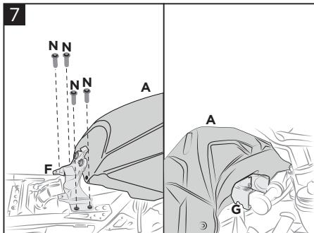
**Mount the Acerbis fuel tank (A), fitting the attachment (G) and fixing the attachment (F) using the original screws (N).**
