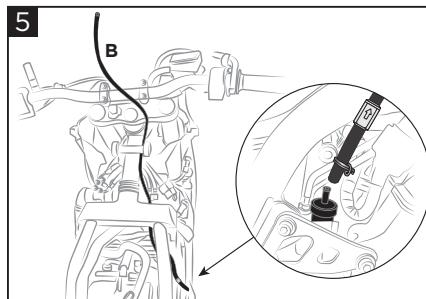
**Attach the cable (B) to the motorcycle and position it as in the figure. Secure by tightening the self-locking clamp (D).**
