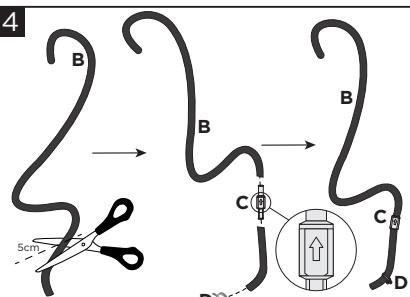
**Cut 5 cm from the tube (B) and join the two parts through the valve (C) with the arrow pointing upward. Insert the self-locking clips (D).**
