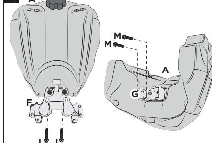
**After disassembling from the original tank the supports (F) and (G), refit them on the tank Acerbis (A), using the original screws (L) and (M).**
