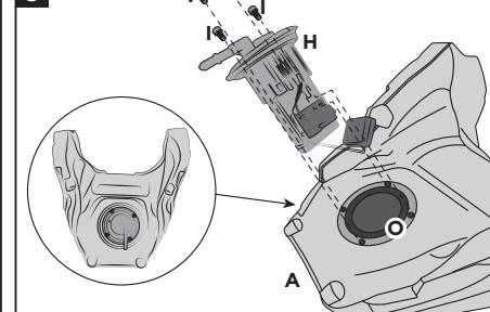
**Remove the pump from the original tank injection (H) and refit it on the tank Acerbis (A), by means of the screws (I) (Torque Max 6Nm) and original gasket. Make sure the connector is facing the towards the rear of the motorcycle (see figure).**
