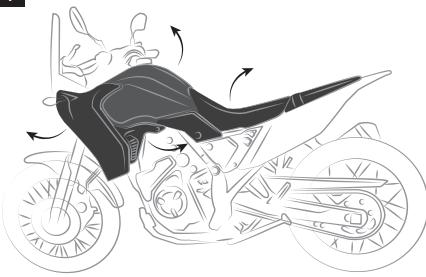
**Remove the orifinal fuel tank by disassembling plastics and seat shown in the figure.**
