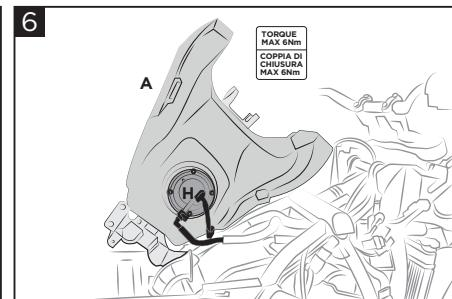
**Connect the connectors to the pump (H) first to mount the tank (A). ATTENTION: when tightening maximum torque spec 6Nm.**
