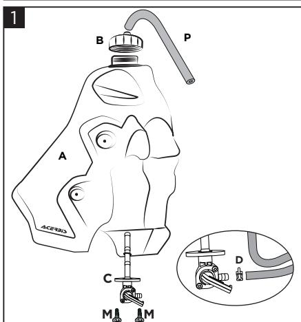
**Insert the tube (P) original in the cap (B). Assemble the petcocks (C) including O-ring using the appropriate screws (M). Fit the original clamp (D) on the pipe before connect it to the petcock.**
