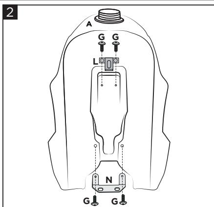
**Fix the bracket (L) through the screws (G). Fix the bracket (N) using the screws (G) without tightening.**
