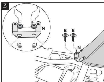
**Insert the rubbers (F) and the bushings (I) in the bracket (N). Place the tank on the frame, making the bracket rest correctly. Fix the bracket (N) through the original screws (E) and tight the screws (G).**
