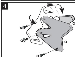
**Reassemble the side panels (O), using the original screws (Q).**
